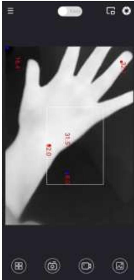
The simple mode requires no additional action and displays the highest, lowest, and center temperatures by default. To view the real-time highest and lowest temperatures in the measurement frame, drag the frame. The measurement frame can be dragged and stretched. To delete the measurement frame, tap anywhere in the frame.
